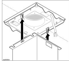
■ Using at least two people, lift the hood and guide the spring clips through their respective slots in the flange at the top of the chimney.
